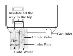
For increased energy efficiency, use pipe insulation. Please install the insulation, according to the illustrations above, making sure to insulate all the way to the top. **Do not** cover any drain or pressure valve(s).
